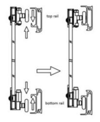
Step B: Please adjust the top roller up and down with the screw shown below using a screwdriver
